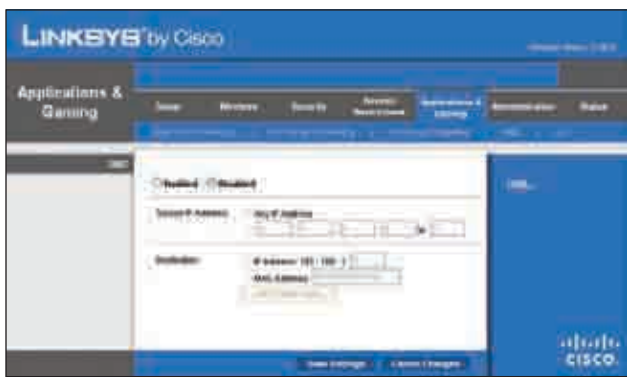
Applications and Gaming > DMZ (Applications et jeux > DMZ)
